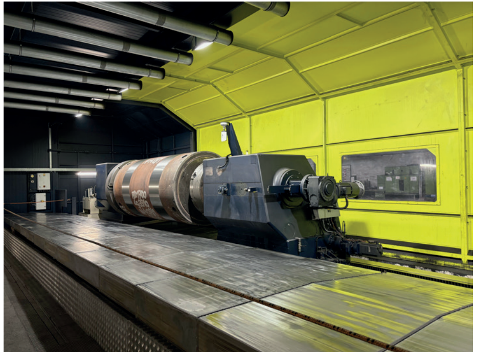
A casting mould inside the closed housing (Picture: Heinrich GEORG GmbH Maschinenfabrik)
