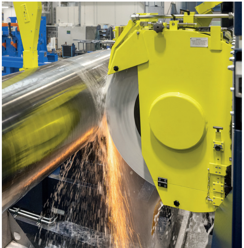
The machine fitted with hydrostatic guides runs exceptionally smoothly, extending the life of the grinding discs (Picture: Heinrich GEORG GmbH Maschinenfabrik)
