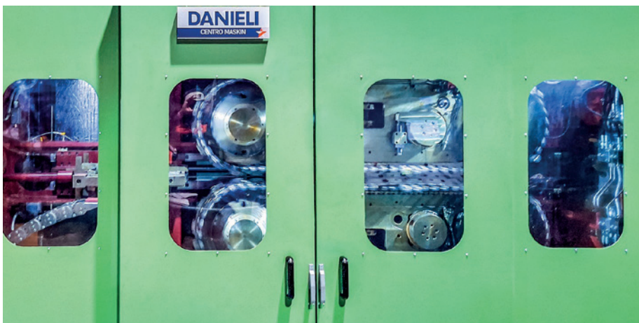
Safely housed high-speed chain-track drawing machine in operation (Photo: Danieli)
