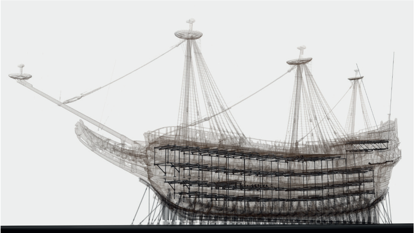
The inner steel skeleton is built as a truss with tubes to stabilize the hull, slow down the movements of the ship and distribute the load (Picture: Alleima)
