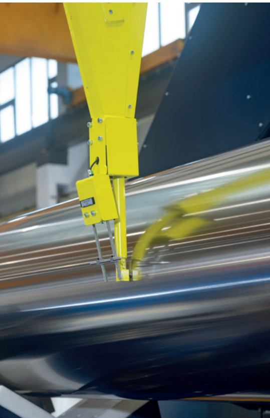
The high-precision 2-point measuring system provides ideal conditions for excellent machining performance (Picture: Heinrich GEORG GmbH Maschinenfabrik)
