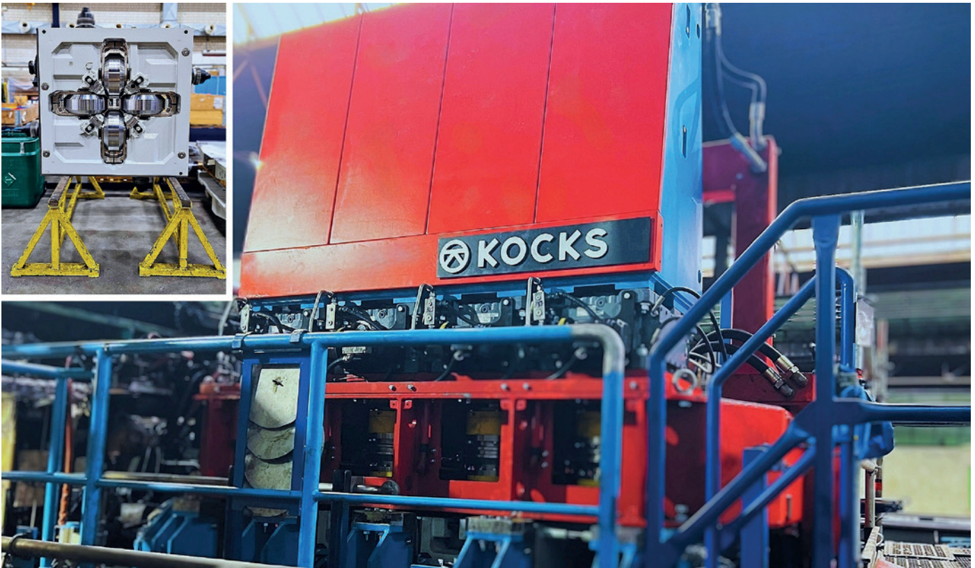
voestalpine Tubulars installed the KOCKS PWW 530/4 rolling unit with four consecutive 4-roll stands (upper left corner) in the hot rolling mill (Pictures: Friedrich Kocks)
