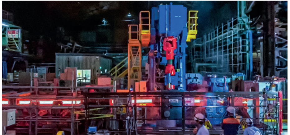
The new roughing mill installed in Nippon Steel's wire rod line (Photo: Danieli)
