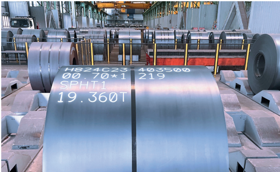
Coils of 0.7-mm-thick strip produced at Shougang Jingtang (Photo: Danieli)
