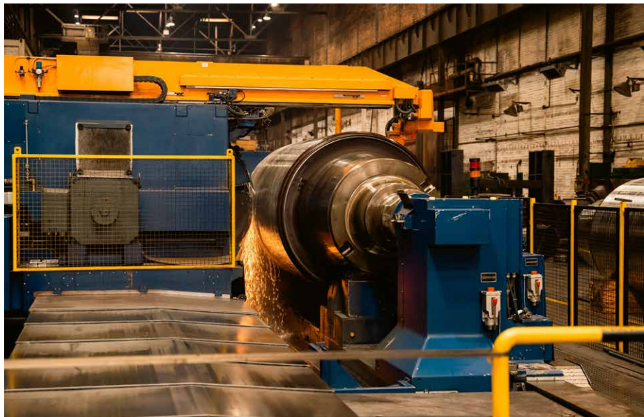
Grinding of a work roll at the SIJ Acoroni hot strip mill (Picture: Weiler Abrasives)
