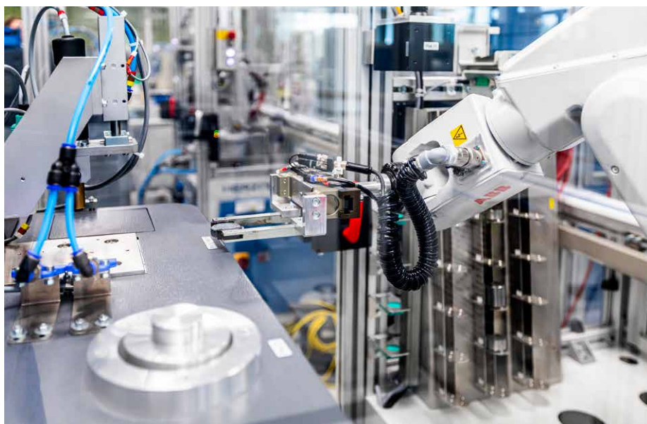
A robot places a steel sample into an OES analyzer (Photo: SSAB/Jaakko Mylly)
