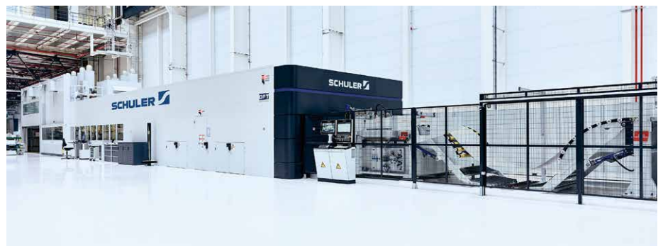
Rosso Steel will be using its new laser blanking line for the cutting of body panels (Picture: Schuler)
