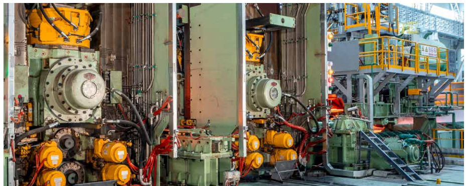
Example of a state-of-the-art two-stand Steckel mill with Steckel furnace (Photo: SMS group)
