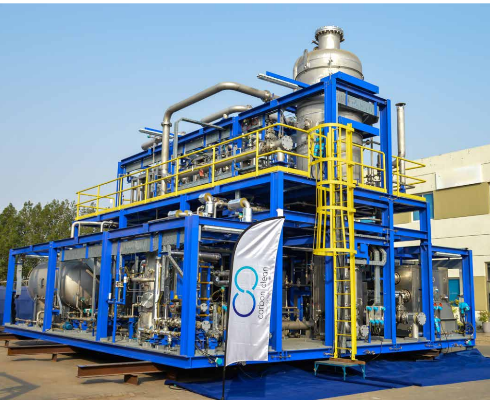
CycloneCC modular technology equipment is ten times smaller in size than conventional CC technologies (Photo: Carbon Clean)
