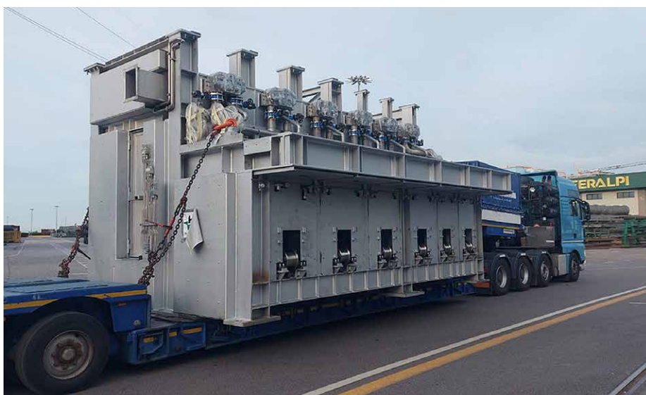
One-piece caster design to minimize the shutdown period (Photo: Primetals Technologies)
