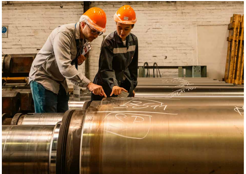
Inspecting work rolls in the roll shop at SIJ Acroni, Slovenia (Picture: Weiler Abrasives)
