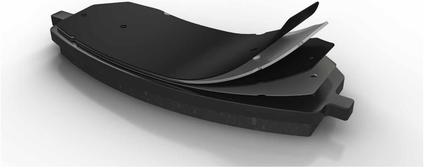
Shims are manufactured by combining different materials, mainly rubber and metal, and attached to the brake pads (Picture: Trelleborg Sealing Solutions Kalmar)
