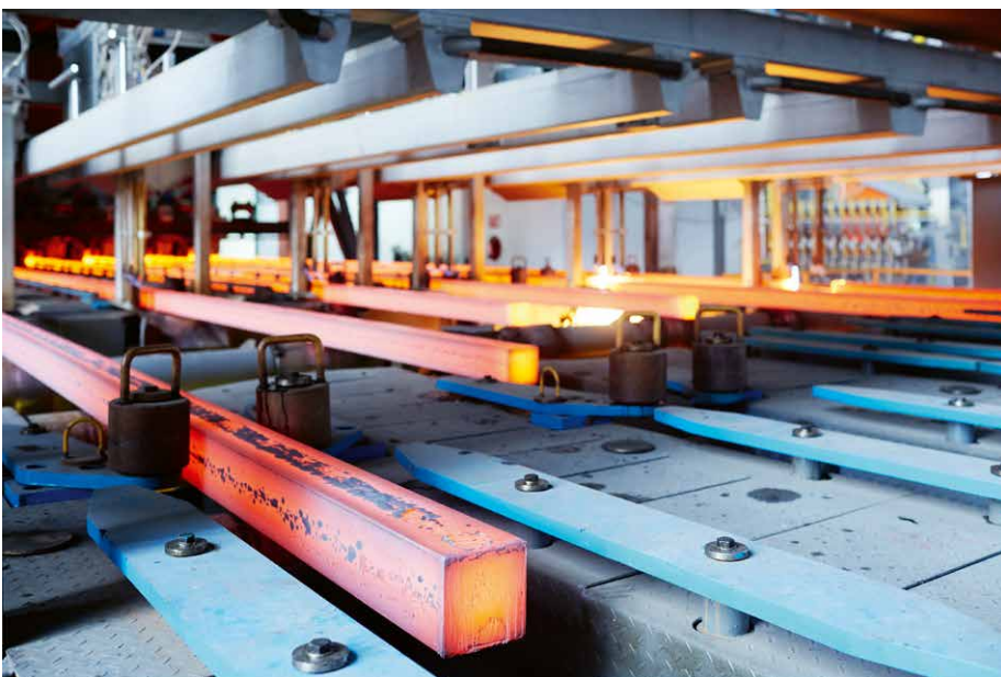
After the upgrade, multi-format caster of Talleres y Aceros will be able to also produce special bar quality (SBQ) steel grades for the automotive industry (Photo: Primetals Technologies)
