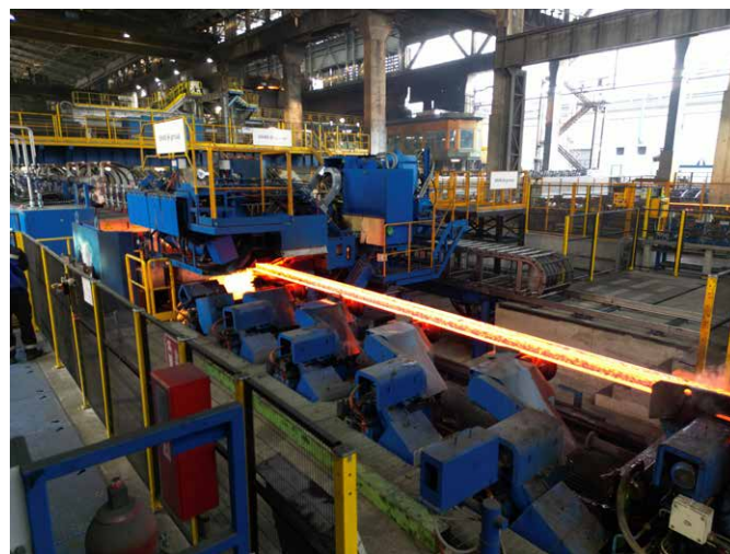
Feralpi Lonato stages 1 and 2 live pictures during production – December 2023: EBROS® billet welding area (Picture: SMS group)
