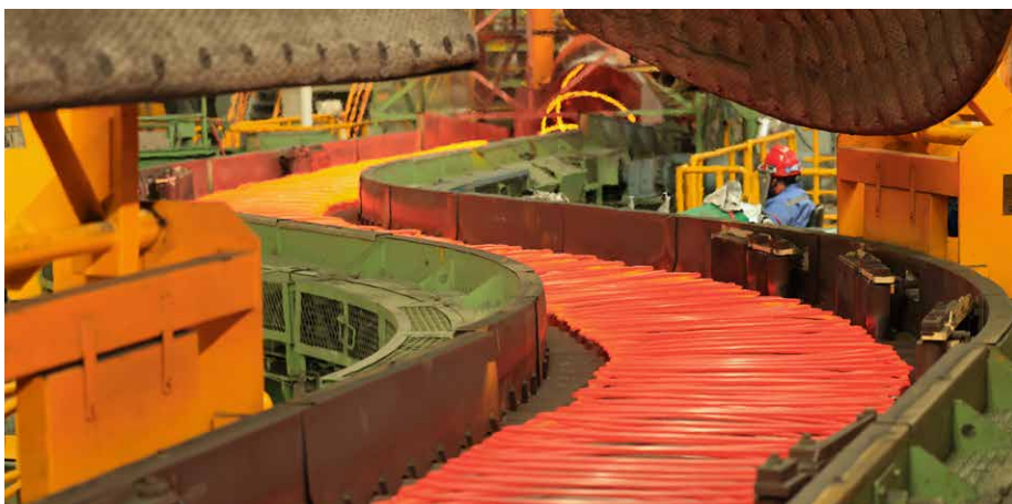
Curved section of the Stelmor conveyor for future in-line direct solution treatment (Photo: Primetals Technologies)
