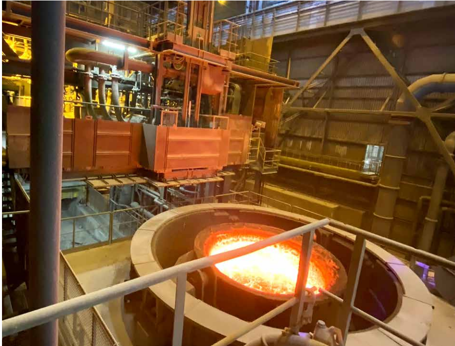
The upgrade of the VD plant to VOD technology will enable Acciaieria Arvedi to produce electrical steel. (Photo: Primetals Technologies)
