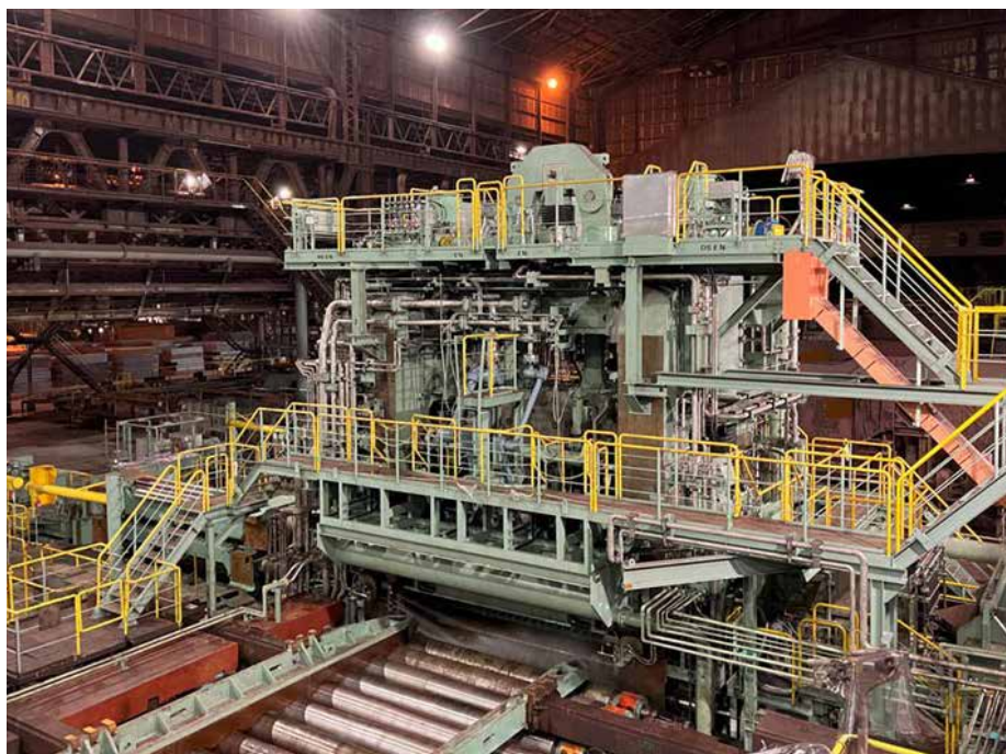
The new plate finishing mill at Kobe Steel's Kakogawa Works (Photo: Primetals Technologies)
