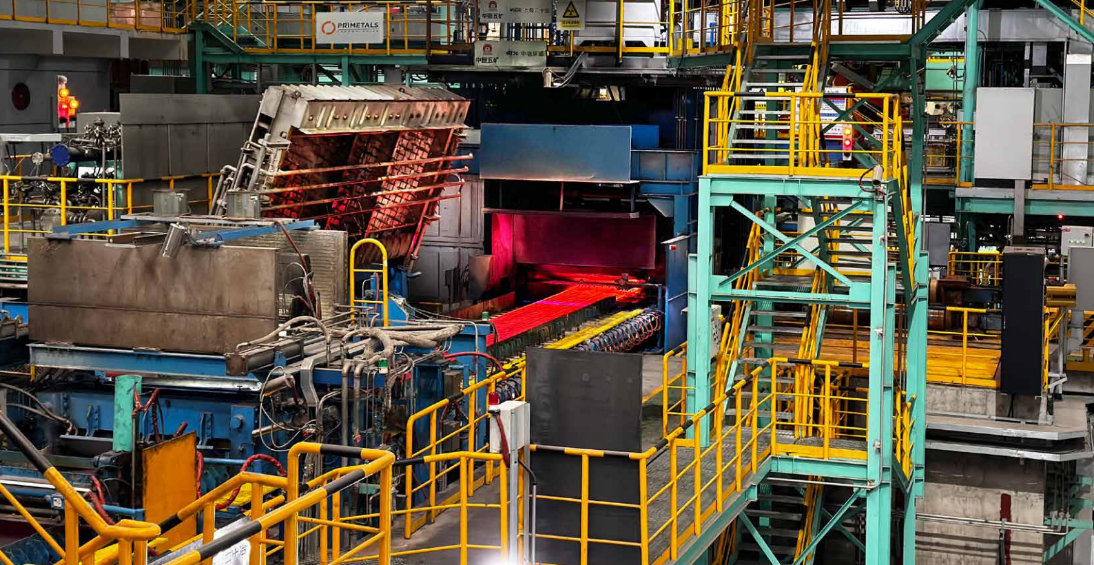
Ultra-compact Castrip casting and rolling plant at Shagang Group's plant in Zhangjiagang, Jiangsu Province, China (Picture: Primetals Technologies)
