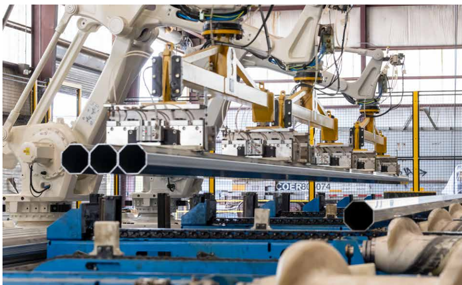
Automatic packaging system of the new OTO tube mill (Photo: Fives)
