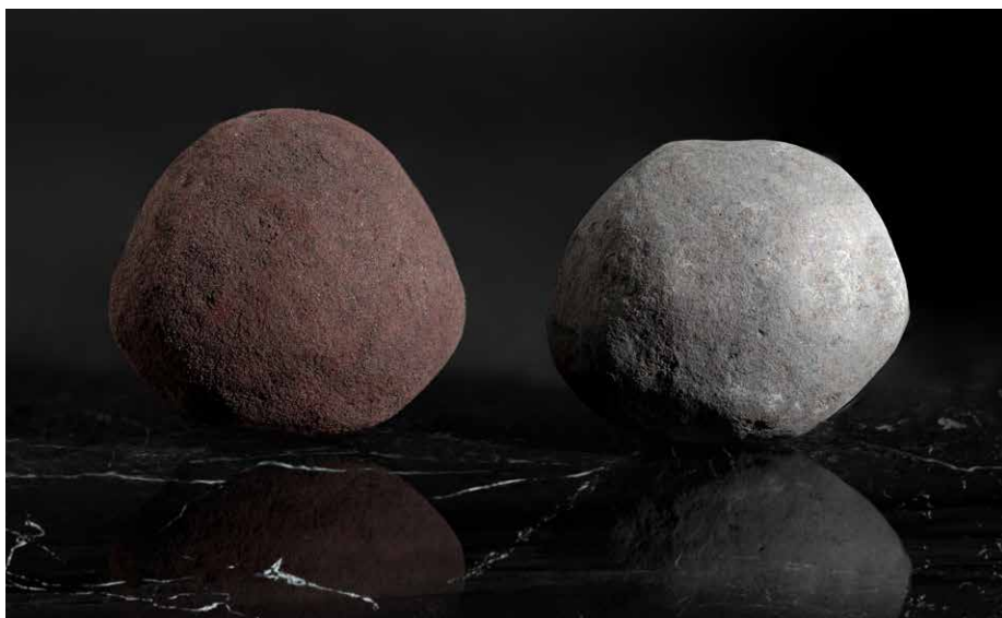
Iron ore pellet (left) and Hydrogen reduced sponge iron from HYBRIT's pilot plant (Photo: SSAB)
