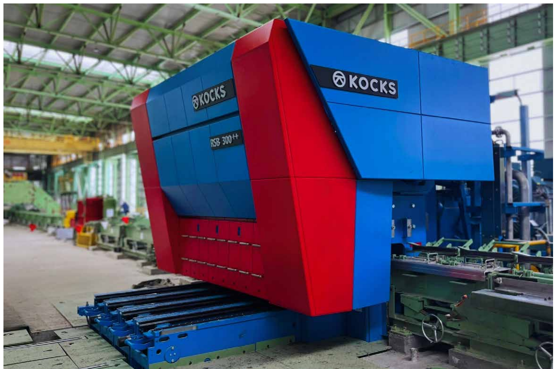
The new reducing and sizing block rolling the first bar at Baosteel (Photo: Kocks)
